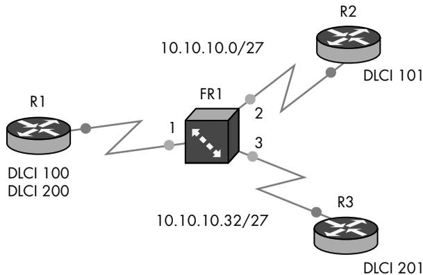
Figure 7-5: Sample hub and spoke Frame Relay network
