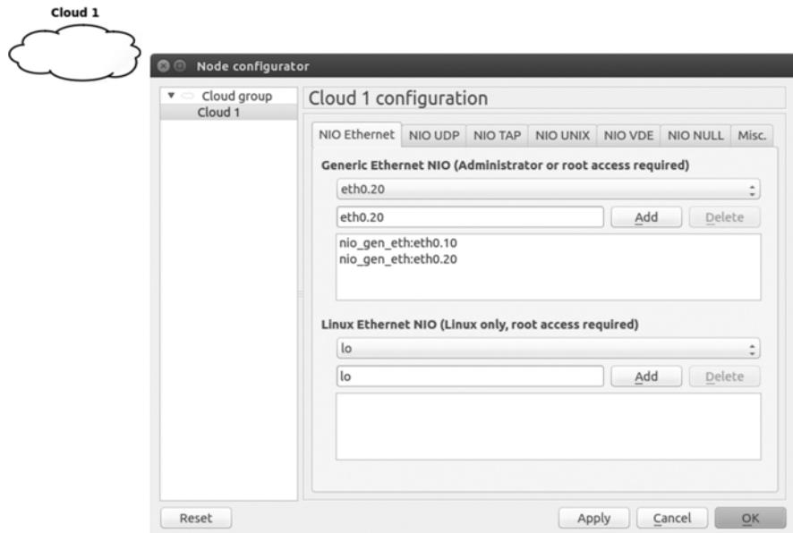
Figure 7-14: Configuring a Cloud node using Linux VLANs
