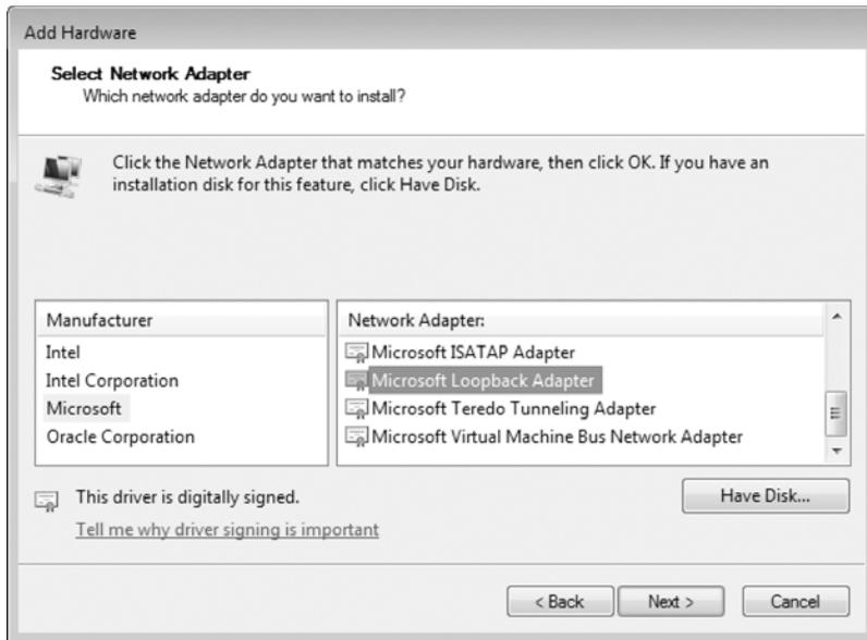
Figure 7-9: Selecting the Microsoft Loopback Adapter
