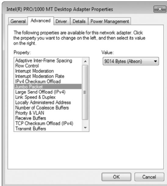
Figure 7-17: Setting the Jumbo Packet size on Windows
