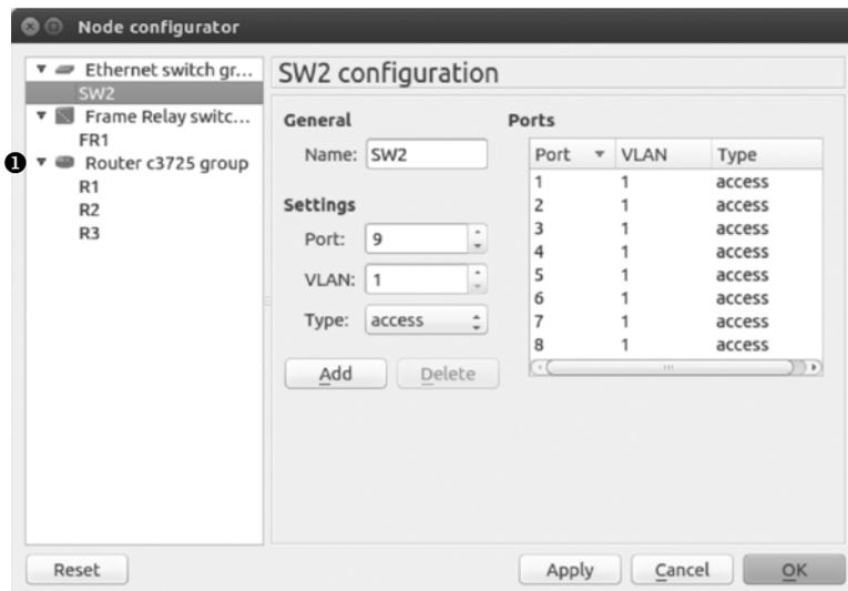
Figure 7-1: Modifying multiple devices using the Node configurator
