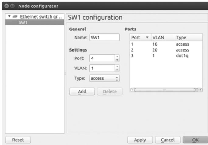
Figure 7-18: Ethernet switch node configured for breakout switch
